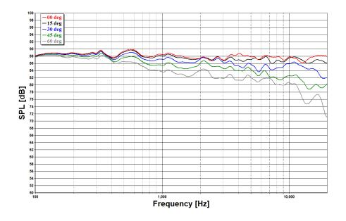
Figure 3: SPL at 1m, 2.83V, on- and off-axis
