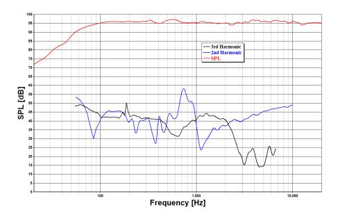
Figure 4: Harmonic distortion at 96dB SPL 1m on-axis
